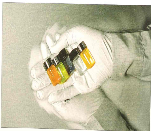
Figure 3b: Solutions of a range of semiconducting polymers with different optical bandgaps and luminescence colours.
